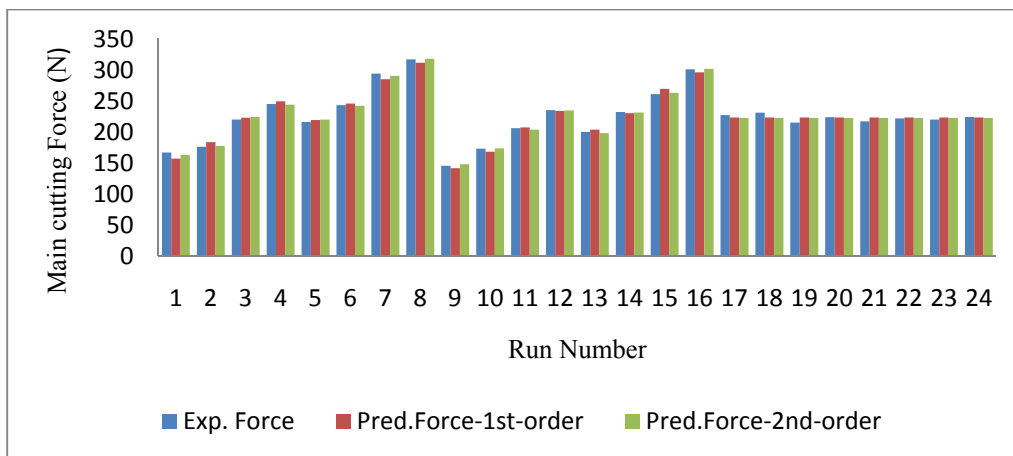
Fig.3. Comparison of measured and predicted cutting force (N)
