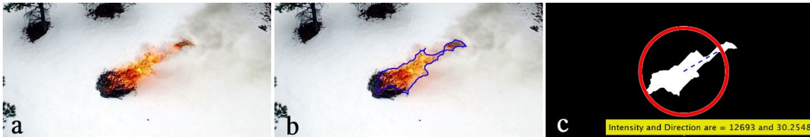
Fig. 4. An experiment result by proposed fire segmentation. a): Original image, b): boundary over segmented part, c): Fire segmentation, intensity, and direction recognition by proposed method (intensity is 12693 pixels and direction are 30 degrees).
