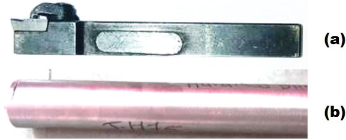
Fig. 3. (a) CBN Cutting Tool (b) Ti6Al4V Workpiece
