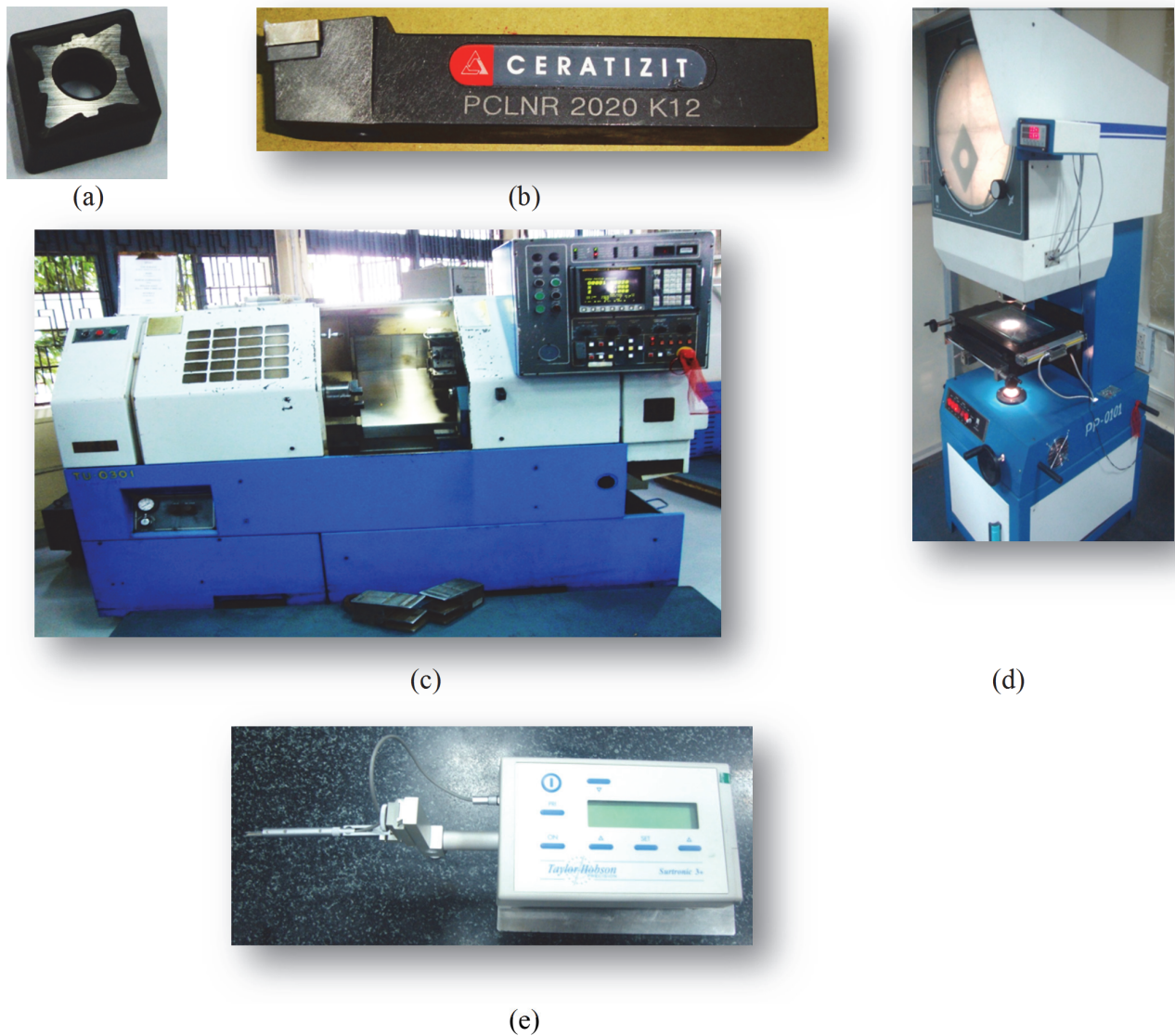
Fig. 4. The components of machining setup (a) carbide insert (CNMG 120408-M5), (b) tool holder (PCLNR2020K12), (c) CNC Lathe (Model LT-16 CNC), (d) Tool Profile Projectors (PP 400 TE) and (e) surface roughness tester (Taylor Hobson, Surtronic 3+).
