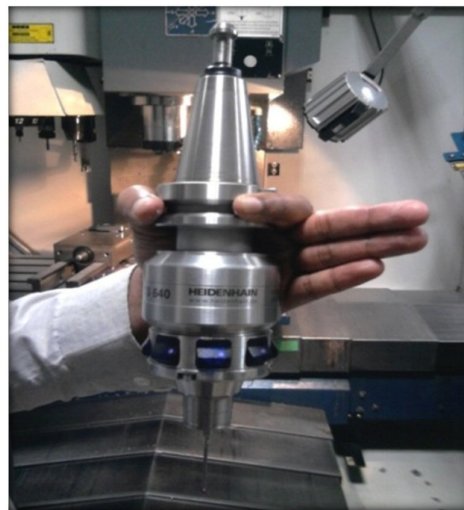
Fig. 4. Touch probe for measuring delamination
