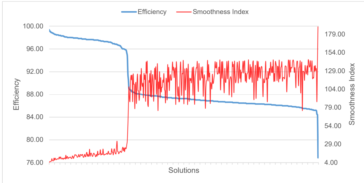
Fig. 3. Line efficiency & line smoothness index values of the feasible solutions
