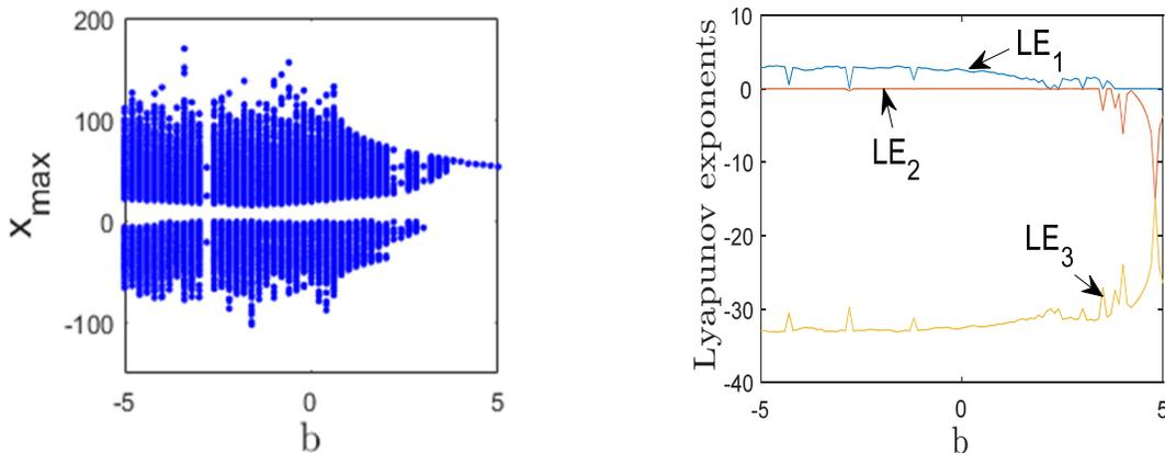
**Fig. 3.** Bifurcation diagram and LEs spectrum of the proposed chaotic system versus parameter  $b$
