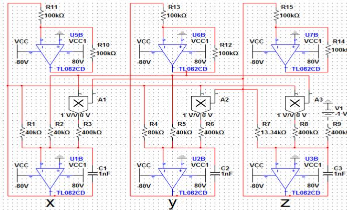
Fig. 6. The schematic circuit of the proposed chaotic system
