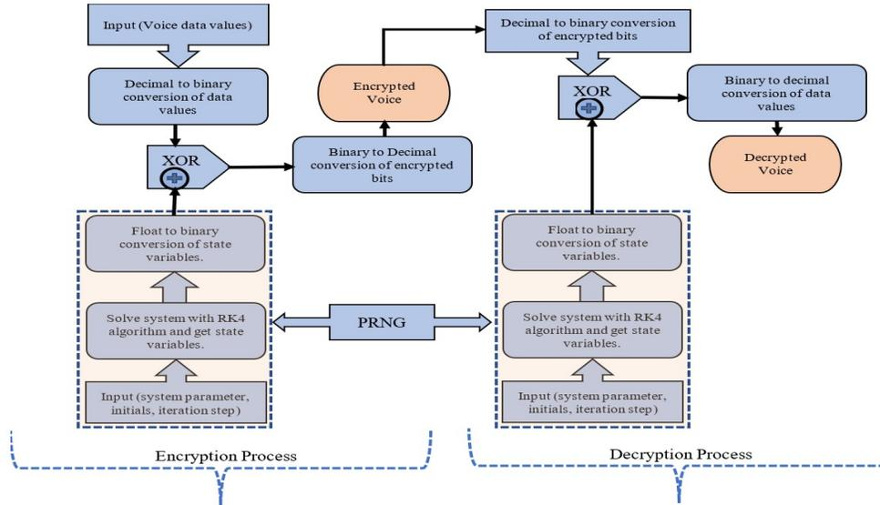
Fig. 9. Flowchart of encryption and decryption
