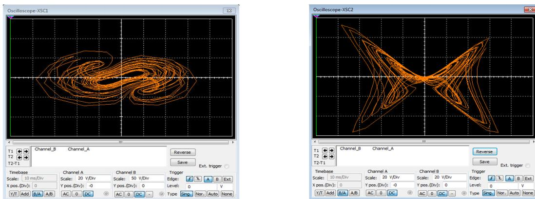
Fig. 7. Multisim outputs of the proposed chaotic system equivalent circuit
