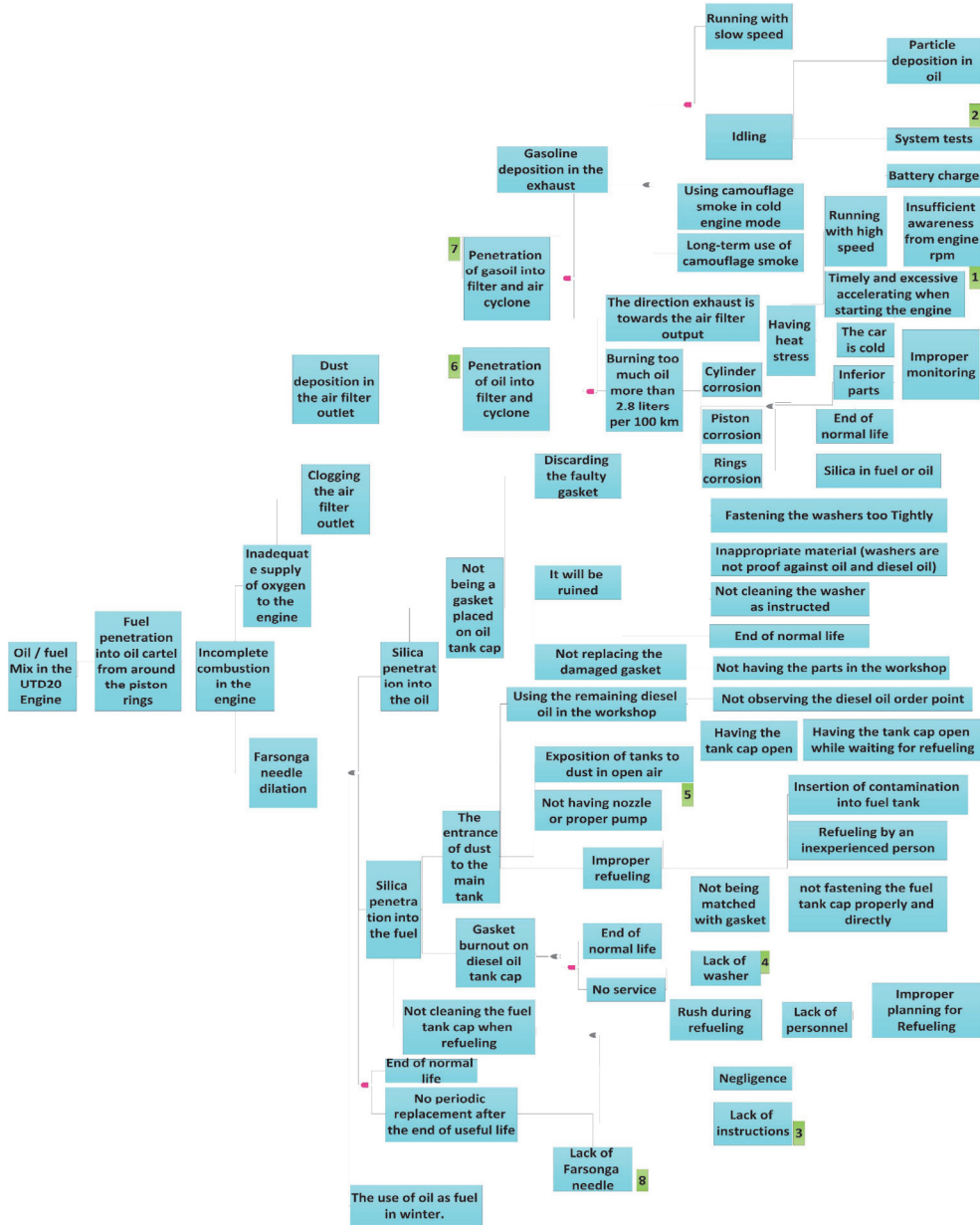
Fig. 2. Network of cause and effect analysis on "mixing oil & fuel" in UTD-20 engine
