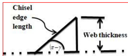
Fig.4 Geometry of the chisel edge
