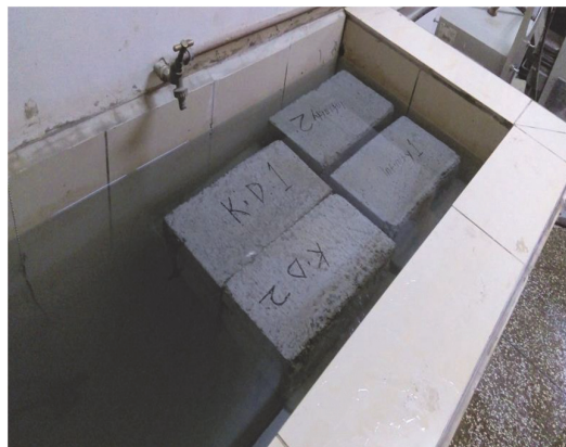
Fig. 2. Block Samples Immersed in Water
