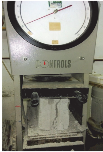
Fig. 3. Block Sample in an ADR Compressive Machine
