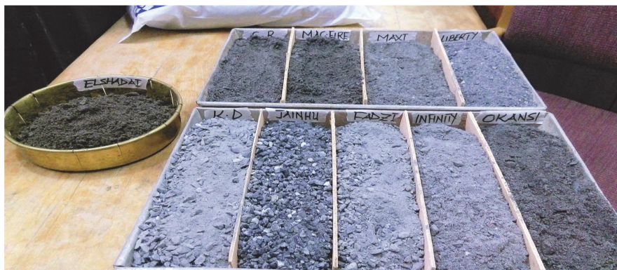
Fig. 1. Samples prepared for oven drying
