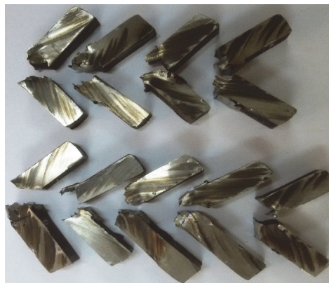
Fig. 5. Fracture surface of toughness test samples with location of fracture.
