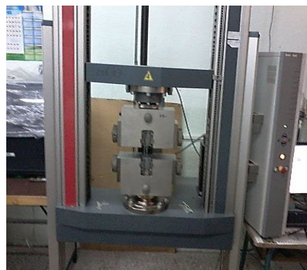
Fig.1. Zwick Roell tensile test machine used for testing
