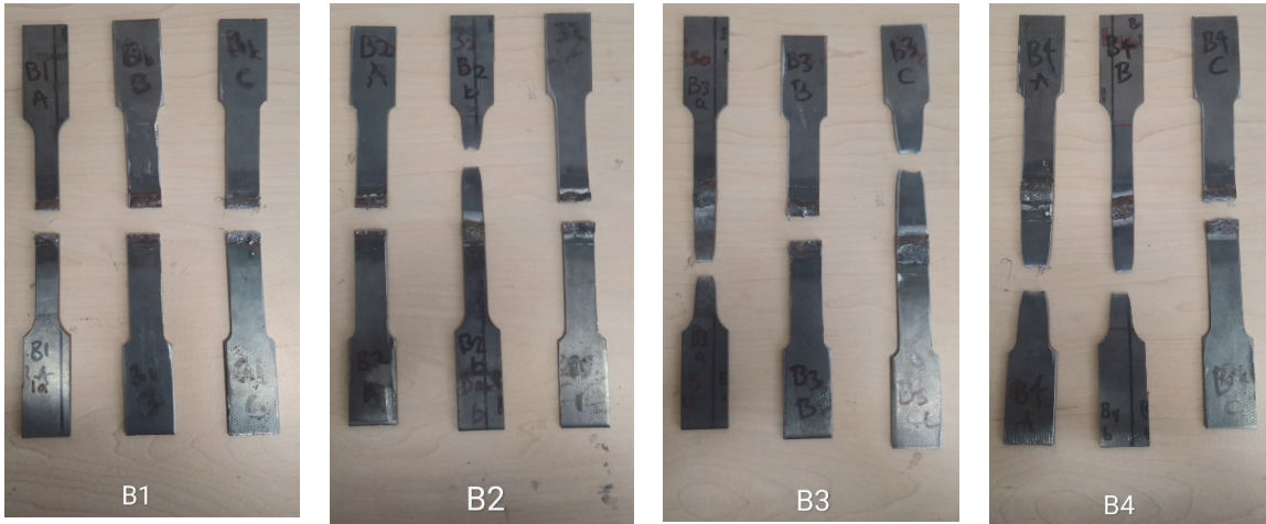
Fig. 6. Failure of Butt Joints due to tensile loading
