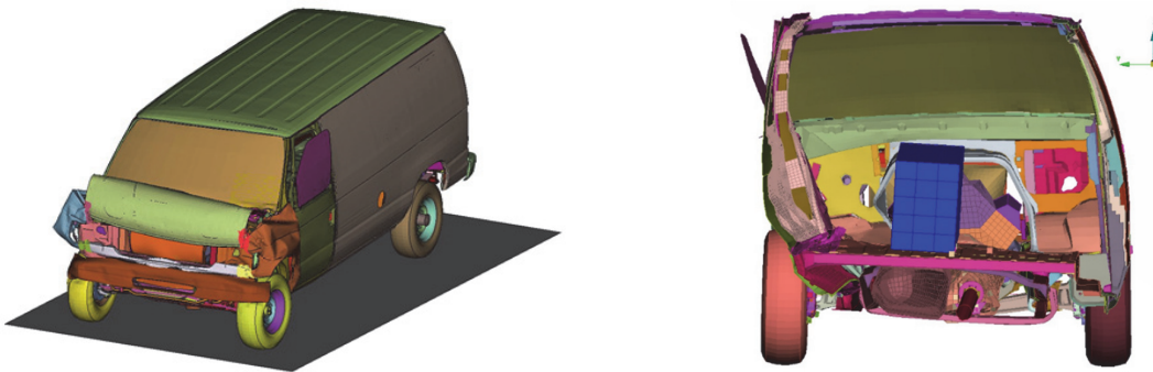
Fig. 8. Front impact (Left Image)/ Side impact (Right Image) based on Euro-NCAP specifications
