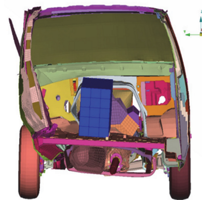
Fig. 25. A view of the Gas tank location after side impact
