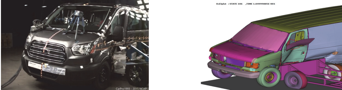
Fig. 9. Side impact test (left image), simulated vs real test (right image)
