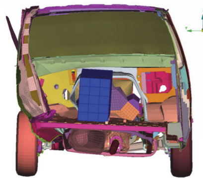
Fig. 48. Side impact- Deformed state- Front view- Some parts of the vehicle are hidden
