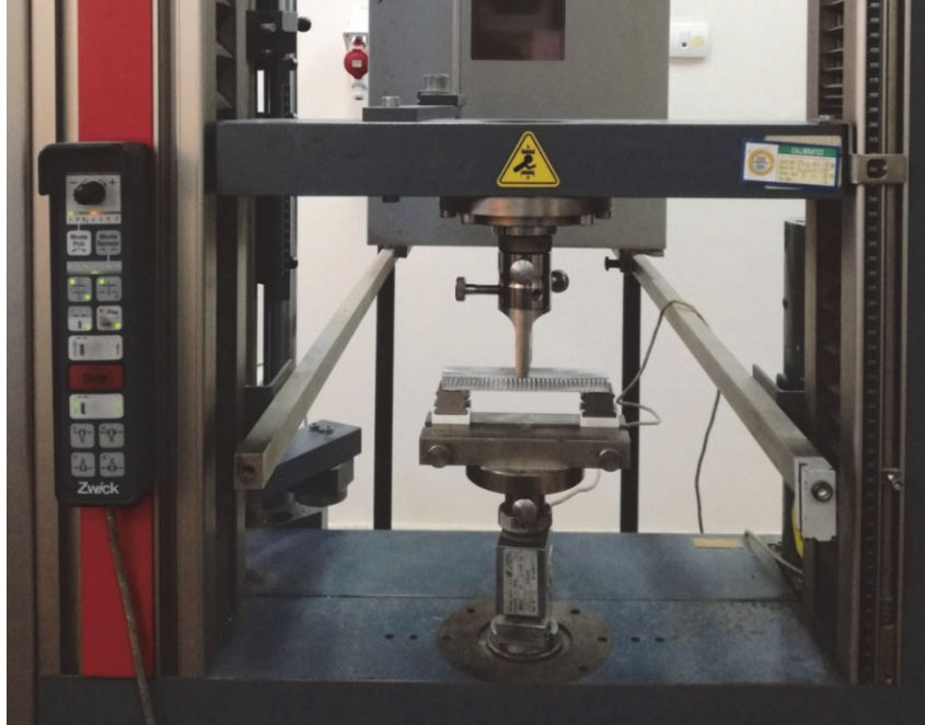
Fig. 8. Three-point bending test setup
