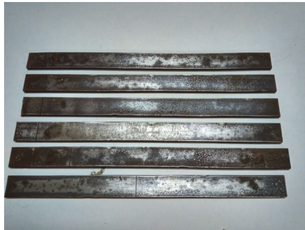
Fig. 4. Cracked beam specimens
