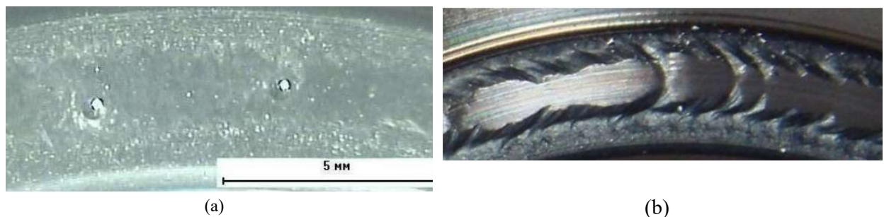
Fig. 3. Surface of annular collar after LTT according to mode #11: a – collar height 2.0 mm, b - collar height 2.5 mm (an attempt of machining of the sample).
