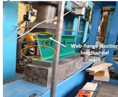
Fig. 11. Failure mode FRP-C-Co 4.
