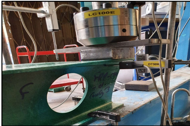
(a) specimens with no opening; seven stub beam specimens with 100 mm diameter circular opening located at the centre; and seven stub beam specimens with rectangular openings, 100 mm wide \times 75 mm deep.
