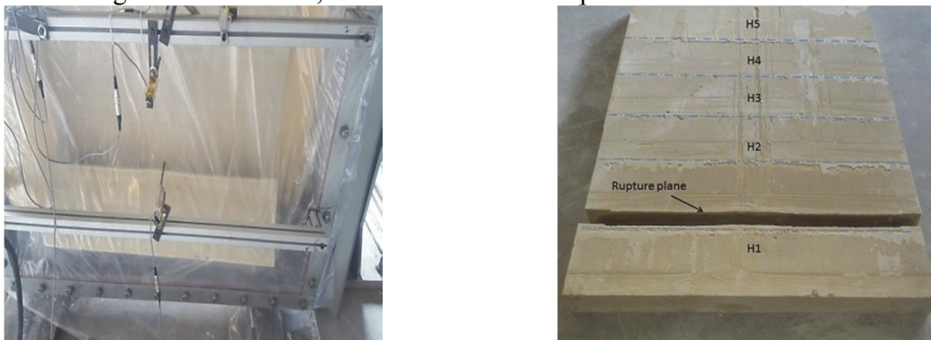
Fig. 10. Typical collapse mode of TS panels at seam H1 under monotonic loading (test series 2)
