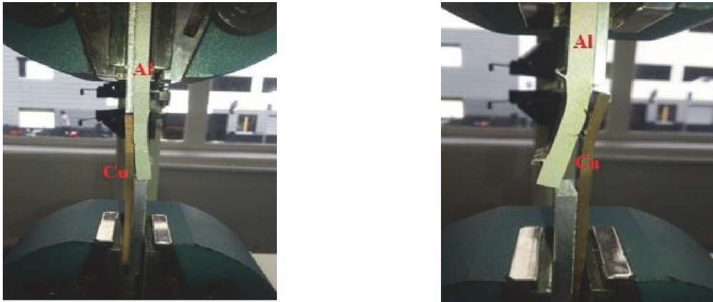
Fig.12. Tensile-shear tested samples of welds made with \omega = 1,400 rpm, v = 60 mm/min and (a) D_p > 0.4 mm and (b) D_p \approx 0.4 mm
