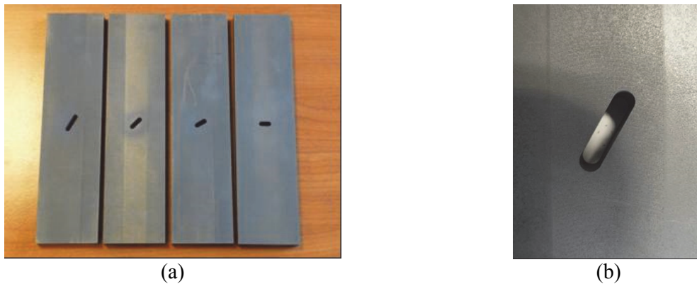
Fig. 1. Views of different inclined U-notches \rho = 2 mm (a); a detail of the notch with \rho = 2 mm, \beta = 60^\circ (b)
