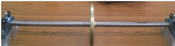
Fig. 2. TGP steel shaft with Aluminium disc
