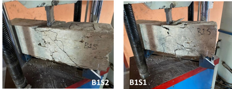
Fig. 6. Damage mode of 50 mm aggregate beam
