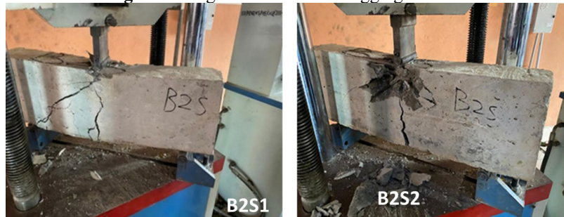
Fig. 7. Damage mode of 25 mm aggregate beam
