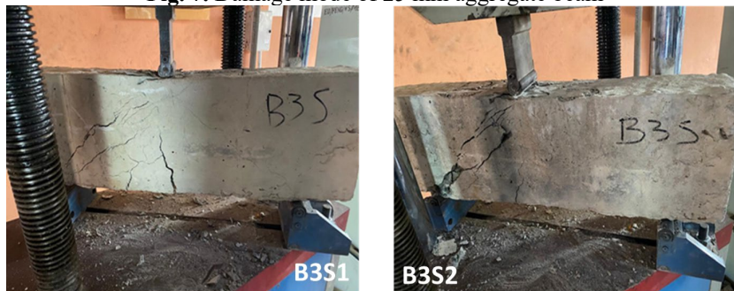
Fig. 8. Damage mode of 19 mm aggregate beam
