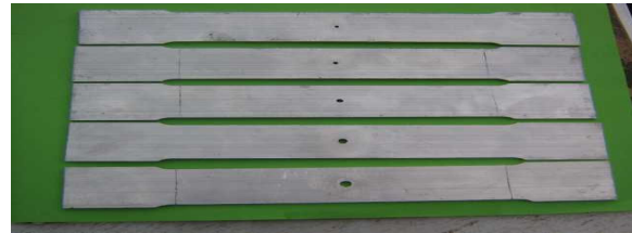
Fig. 2. Specimens pierced with diameters (1-2-3-4) mm
