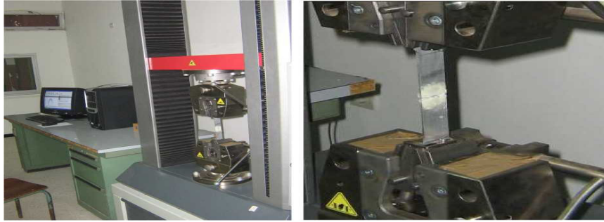
Fig. 5. View of the Specimen Positioned Between the Machine's jaws
