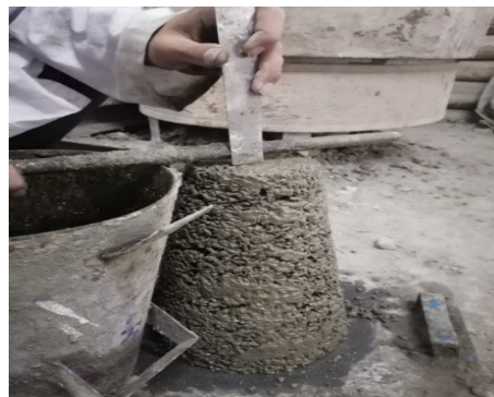
Fig. 2. Slump test on concrete mix Slump Test on Concrete
