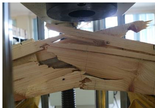
Fig. 2. Damage to the connection on the CLT test object
