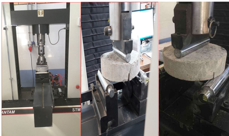
Fig. 4. Different loading modes for the ENDB specimens
