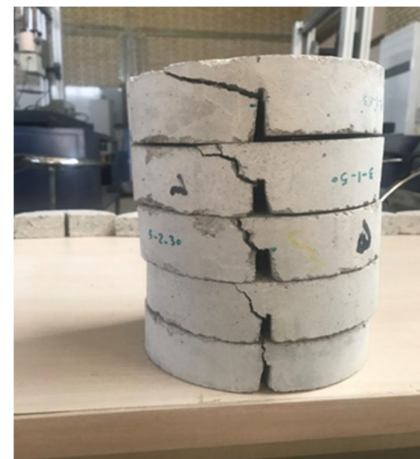
Fig. 5. Fracture paths of ENDB specimens in pure and mix mode I/III
