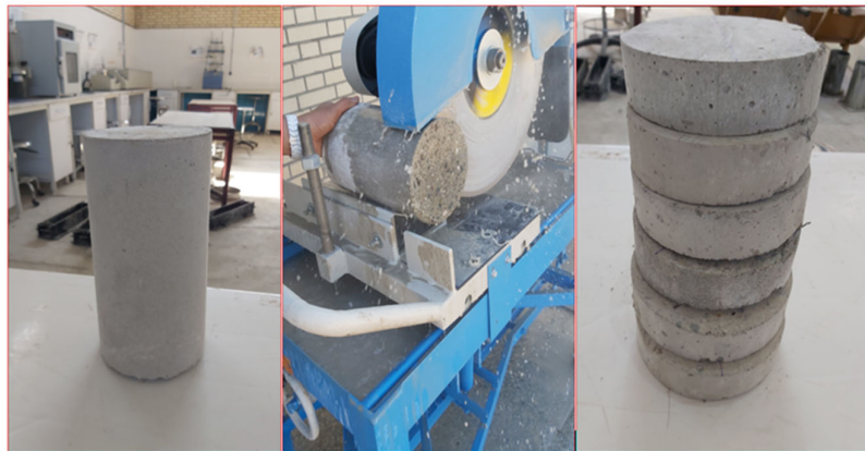
Fig. 3. Steps of preparation and cutting of disc shape specimens
