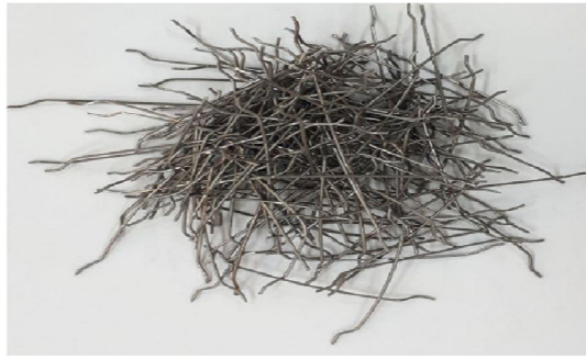
Fig. 2. Hooked end steel fiber
