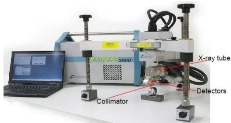
Fig. 9. XRD stress analyzer device
