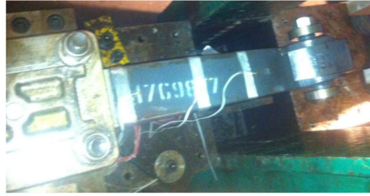
Fig. 12. Strain gauge on leaf spring
