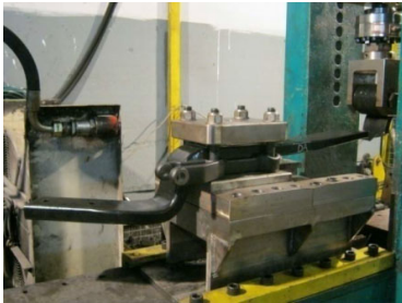
Fig. 7. Pre-loading of Z type leaf spring
