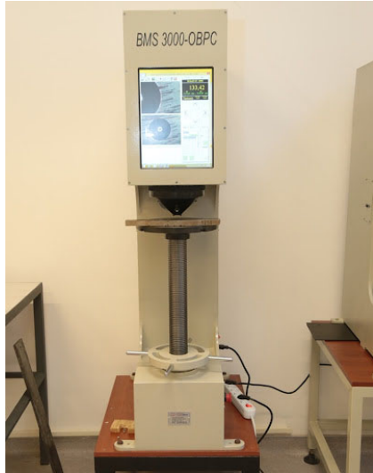
Fig. 10. Brinell hardness test device
