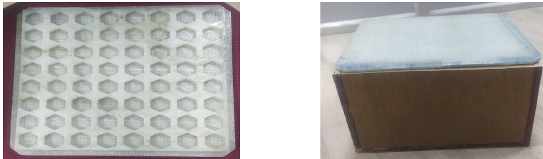
Fig. 12. GFRP Hatch cover model
