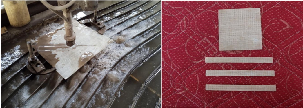
Fig. 4. Working of water jet machine and the result
