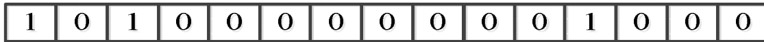
Fig. 1. The basic structure of an answer to a problem of locating the emergency units
