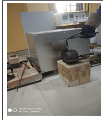
Fig. 2. Pouring the molten metal into the die
