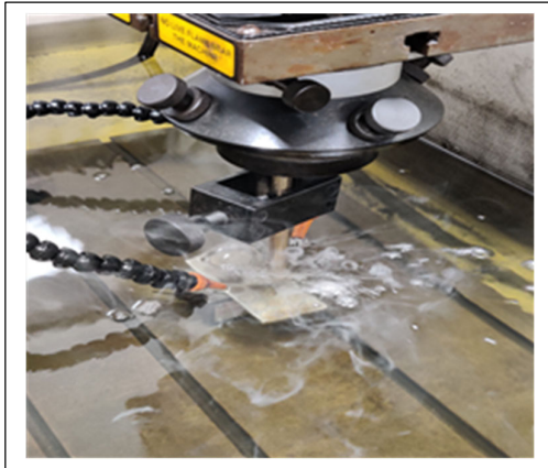
Fig. 3. Schematic showing Machining in EDM
