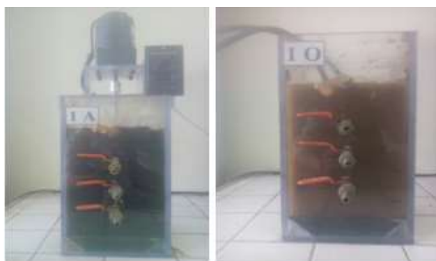
Fig 9. Anaerobic tanks and SBR used in the study
